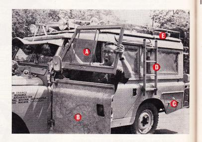
explain our routes to visitors. Since the Rover's interior was also modified, we had to cut an access door (C) to the tool compartment. Short magnesium ladders (D) carried on the sides can be joined as one ladder, or used to obtain additional traction in mud, snow, or sand. Large spare parts, such as a spring, were fastened to roof rack (E).
